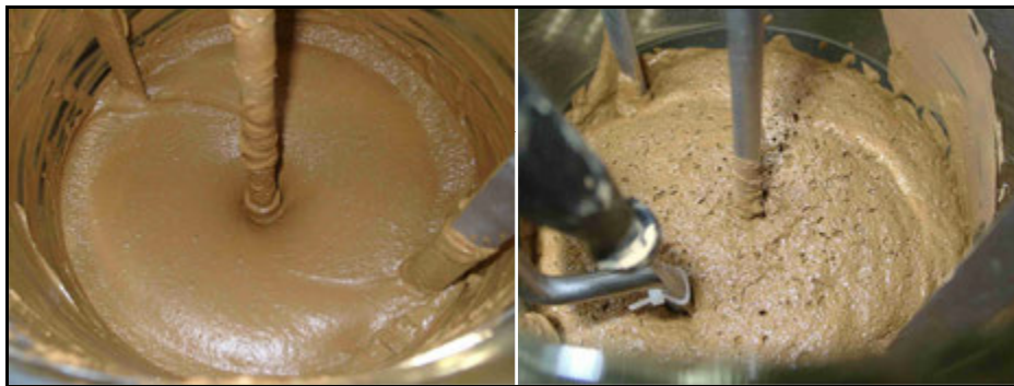
Figure10: Gassing at increased viscosity (left ungassed slurry).
