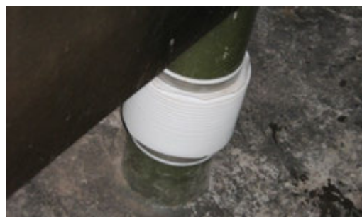
Figure 6: PTFE bellows installed at Ezulwini for aqueous weir height adjustment
