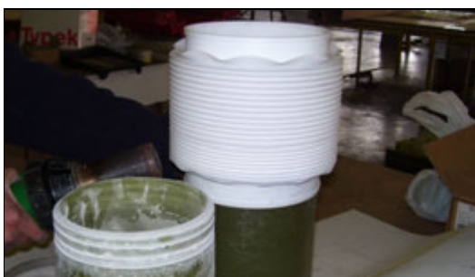
Figure 6: PTFE bellows installed at Ezulwini for aqueous weir height adjustment
