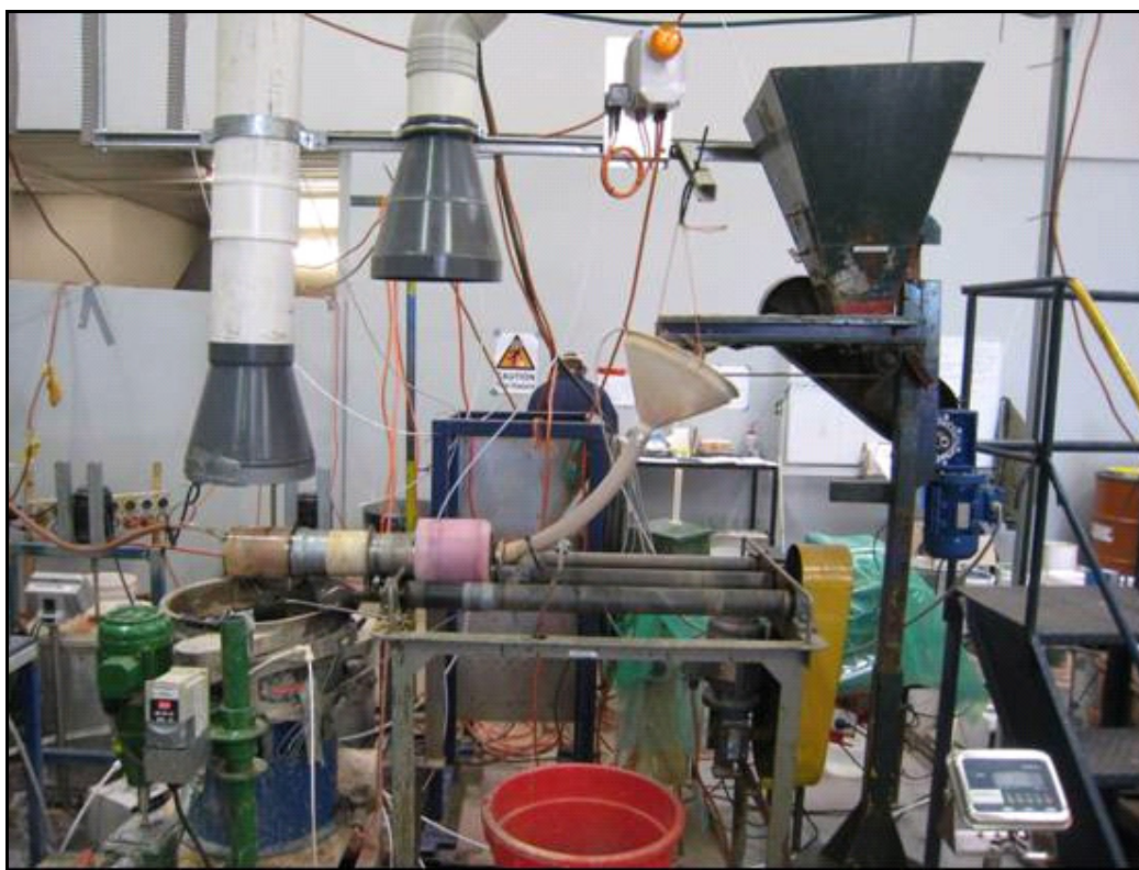
Figure 2: Run 1 Scrubber and Kason Screen 1 Configuration
