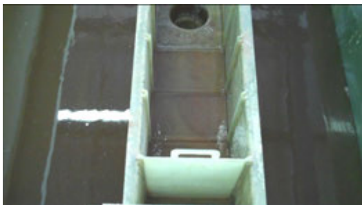
Figure 5: Aqueous overflow weir, showing guides for aqueous splitter plate (inserted)
