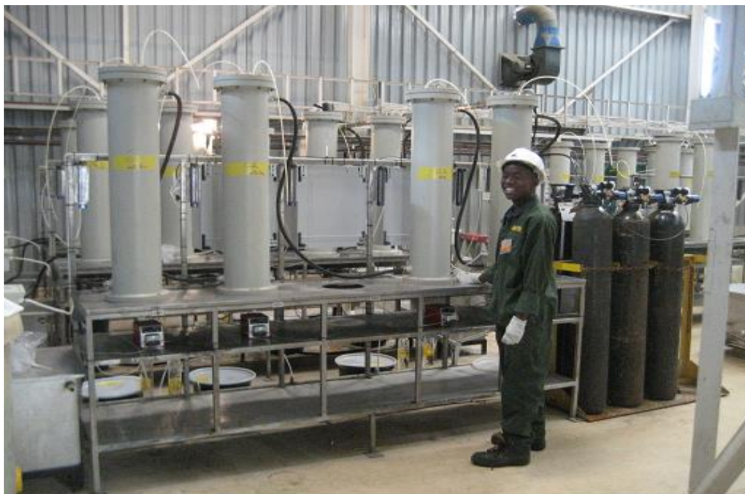
Figure 1: 1 m Column Set-up
