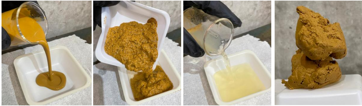
Figure 6: (left to right) Re-slurried composite sample CP008. Re-slurried sample flocculated with Magnafloc 1101. Resultant centrifuge Centrate. Resultant centrifuge cake.
